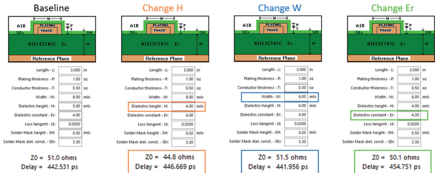
Figure 23. PCB microstrip examples.
