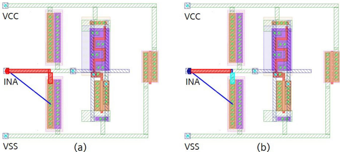
Figure 3: Debugging resistance violation of an ESD path in a simple circuit design with ESD protection on I/O pad. (a) All polygon segments with a resistance violation are highlighted in red; (b) Polygon segments with a resistance violation are highlighted in different colors based on the percentage contribution of each polygon to the total effective resistance of the ESD path.
