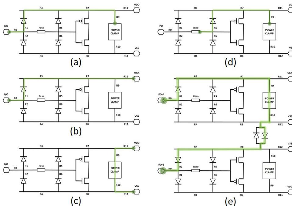
Figure 1: Common ESD protection schemes and ESD discharge paths (highlighted in green): (a) I/O pad and power clamp; (b) I/O pad and power pad; (c) power pad and ground pad; (d) ESD resistor and power clamp; (e) I/O pad and I/O pad [3, 4].
